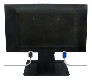
After attaching all necessary cables to your monitor and computer, (See Connecting Your Monitor for cable attachment,) use the cable management slot to organize all cables as shown above.
